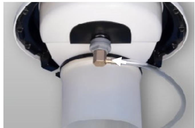
To do this, cut the old hose through the service flap over the hose nozzle of the angled hose connection using a cutter so that you can pull it off.
