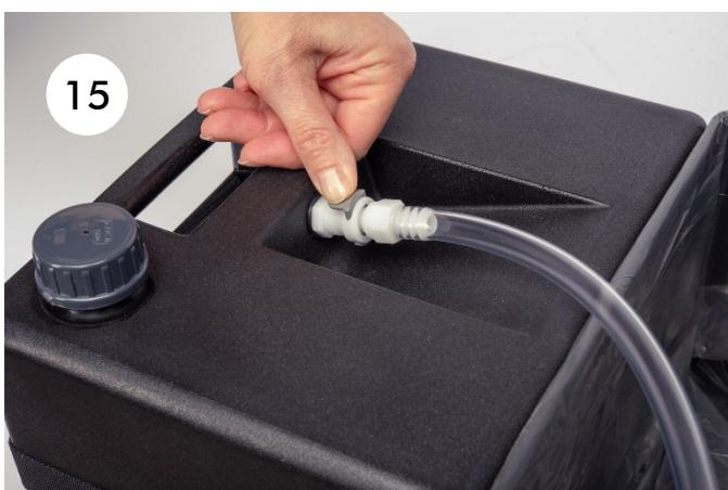
15. Pull the hose with the plug out of the hose connection by pressing down the release button on the hose connection.
