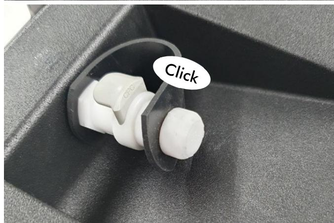
16. Close the hose connection for transporting the liquid tank by pressing in the stopper attached to the cassette with the stopper holder until you hear it click into place.
